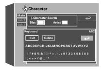
**4.** Press the cursor button to move the cursor on the OSD screen to the "**Keyboard**" area, then move the cursor on the desired character and press the **ENTER** button.
